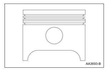
2. Using the Feeler Gauge Set, measure the piston ring-to-groove clearance.
